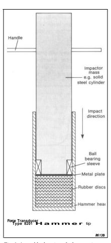
Fig. 3. Assembly drawing of a large impactor using the Briiel & Kjcer Force Transducer Type 8201
