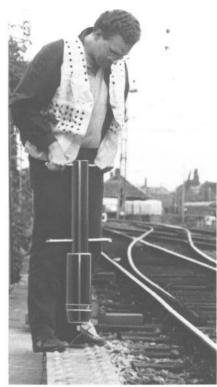
Fig. 6 The operator excited the structure by applying an impact to a small rubber patch placed on the structure
