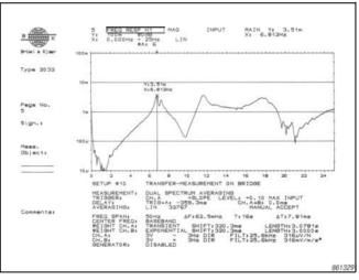
Fig. 8. A typical frequency response function obtained by the test
